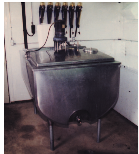
210 gallon bulk tank
