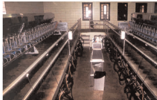
Two x 24 indexing stanchion (Casse system) low pipeline (Old Chatham, New York).
