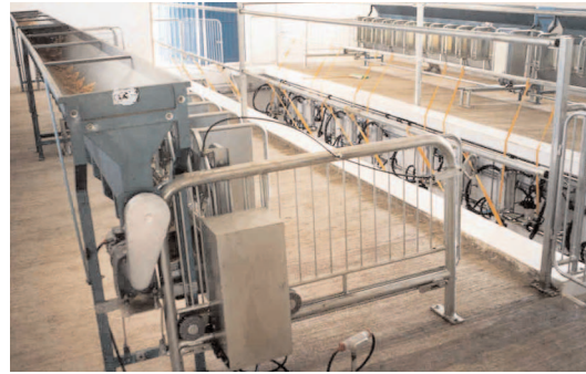
Two x 24 indexing stanchion (Casse system).
