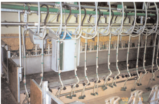
New Casse system with automatic take-off and automatic swing-over.
